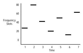
FIGURE 7. FREQUENCY HOPPING SPREAD SPECTRUM
