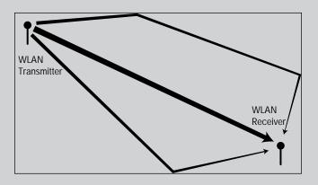
Figure 9. Radio Signals Traveling over Multiple Paths
